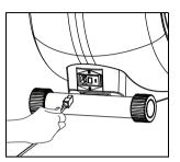
2. Plug the other end into a grounded outlet so you can maintain a consistent power source without overloading any other circuitry. Be sure to use the appropriate voltage. Refer to *Grounding Instructions* in the owner's manual.
